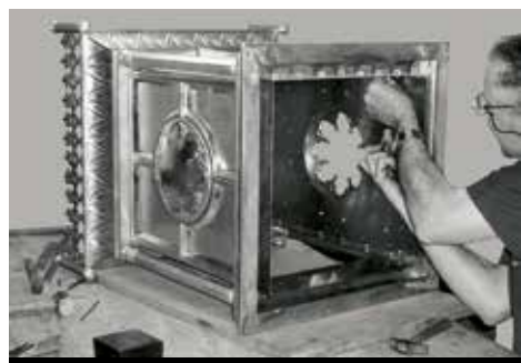
Mounting and adjusting of all the engraved panels, doors and other fittings. It is essential to execute this phase with the utmost perfectionism to ensure a quality product. The tabernacle is after taken apart once again and carefully polished & plated.
